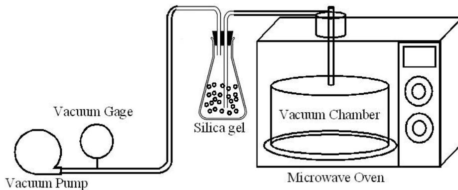
**Figure 2.** Experimental setup of microwave vacuum drying.
