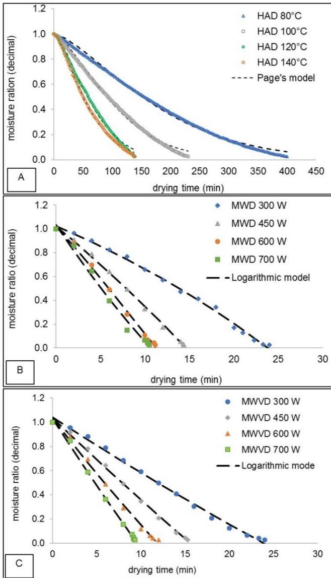
**Figure 3.** Changes in moisture ratios at different drying methods for (A) hot air at 80 - 140°C, (B) microwave drying at 300 - 700 W, and (C) microwave vacuum at 300 - 700 W.
