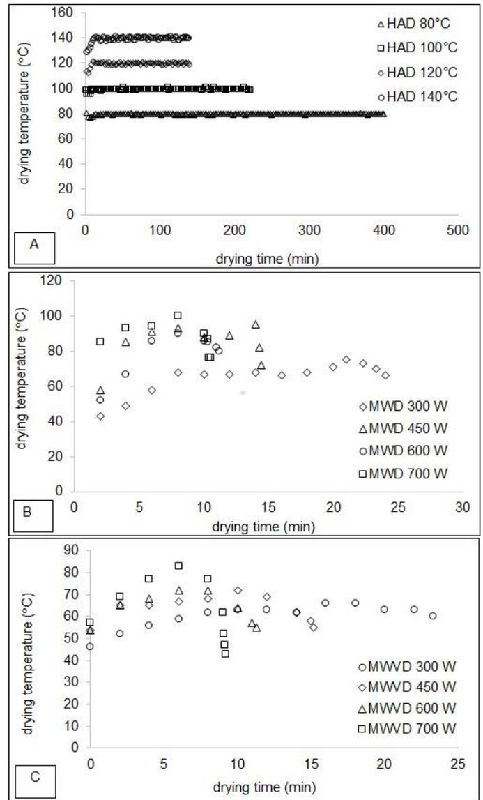
**Figure 4.** Changes in temperatures at different drying methods for (A) hot air at 80 - 140°C, (B) microwave drying at 300 - 700 W, and (C) microwave vacuum at 300 - 700 W.
