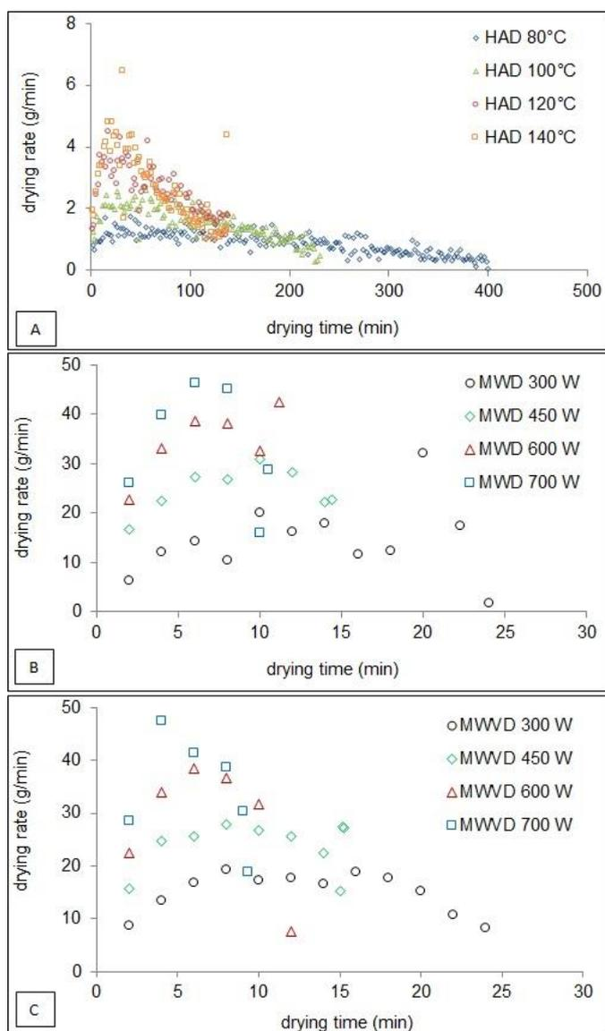
**Figure 5.** Changes in drying rates at different drying methods for (A) hot air at 80 - 140°C, (B) microwave drying at 300 - 700 W, and (C) microwave vacuum at 300 - 700 W.
